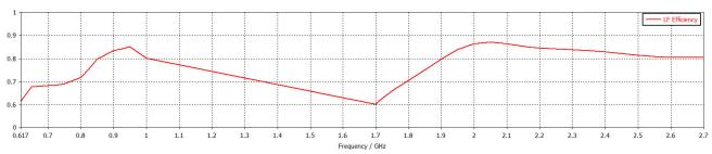
\*Efficiency simulated in CST Microwave Studio excluding cable loss.
