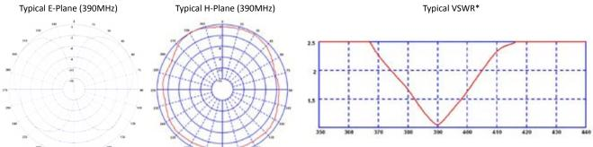
\*measured with AUGHB-S1 mounted on a 600x600mm (19.7' x 19.7') groundplane with 5m of CS23 cable.
