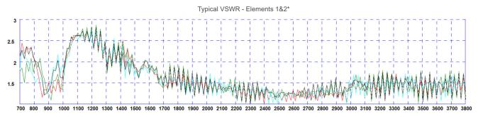
\* VSWR measured with 3m (10') of RG174 cable Green and Red Plots = Elements 1&2 in free space Black and Blue plots = Elements 1&2 on a 400x400mm ground plane
