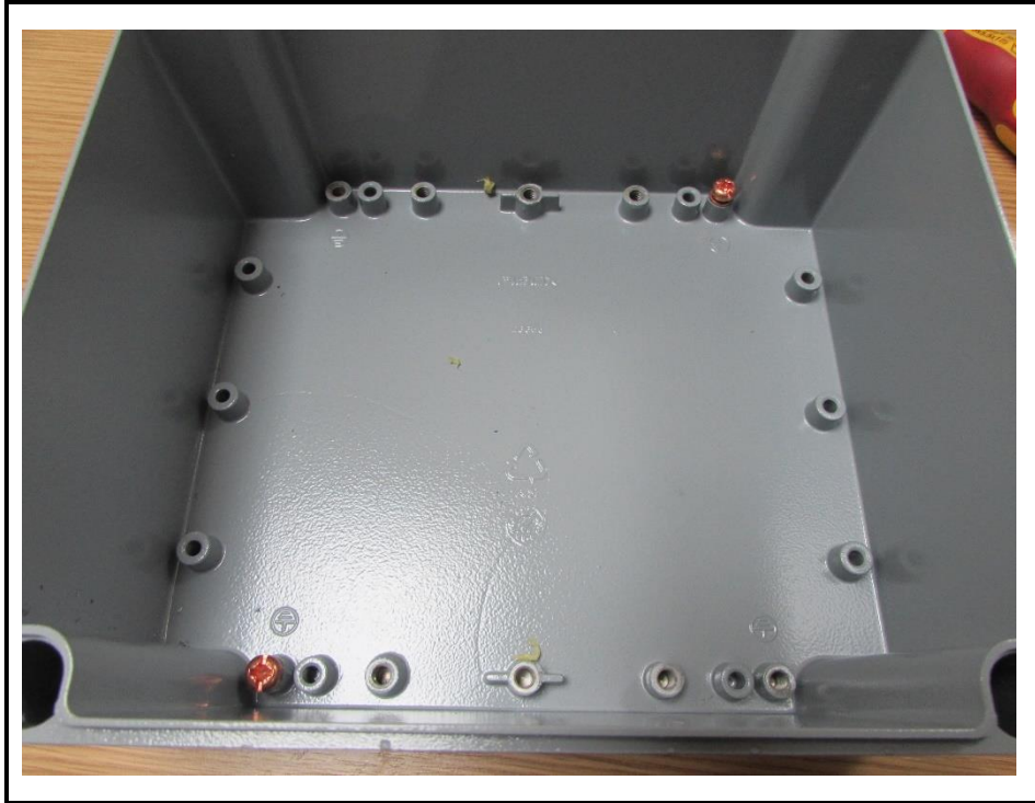
Figure 5: Post Test Photos – IPx9K Water Ingress
