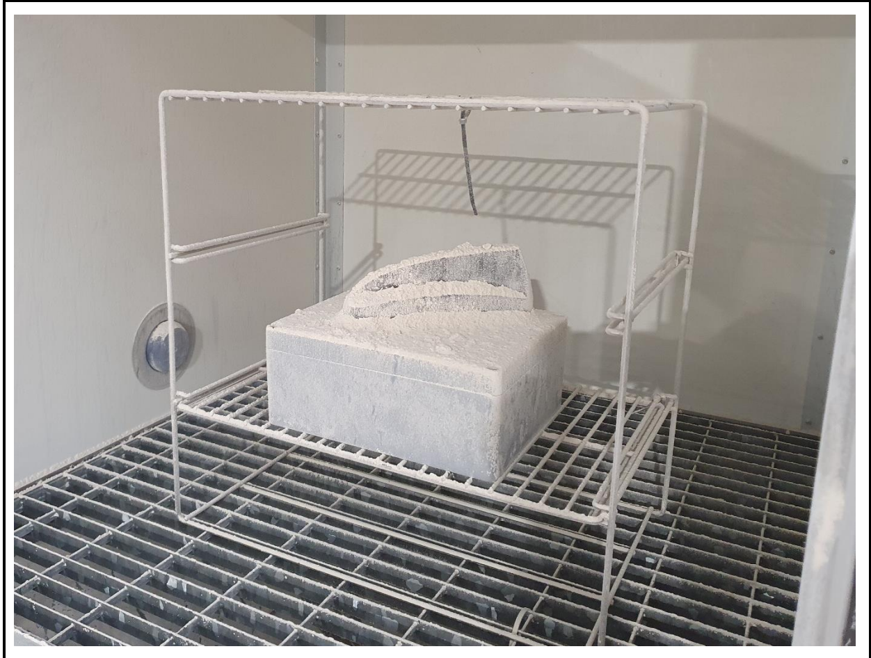
Figure 1: Test Item Orientation: IP6Kx Dust Ingress
