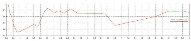
\* Efficiency simulated in CST Microwave Studio with 175mm (7") cable
