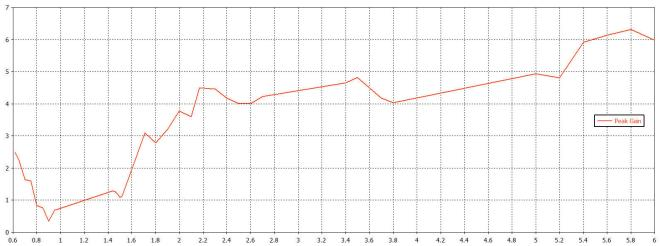
\* Peak gain simulated in CST Microwave Studio with 175mm (7") cable
