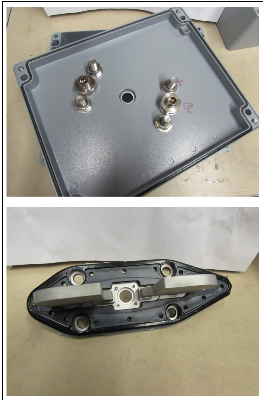
Figure 3: Post Test Photos – IPx9K Water Ingress TRNM[G]
