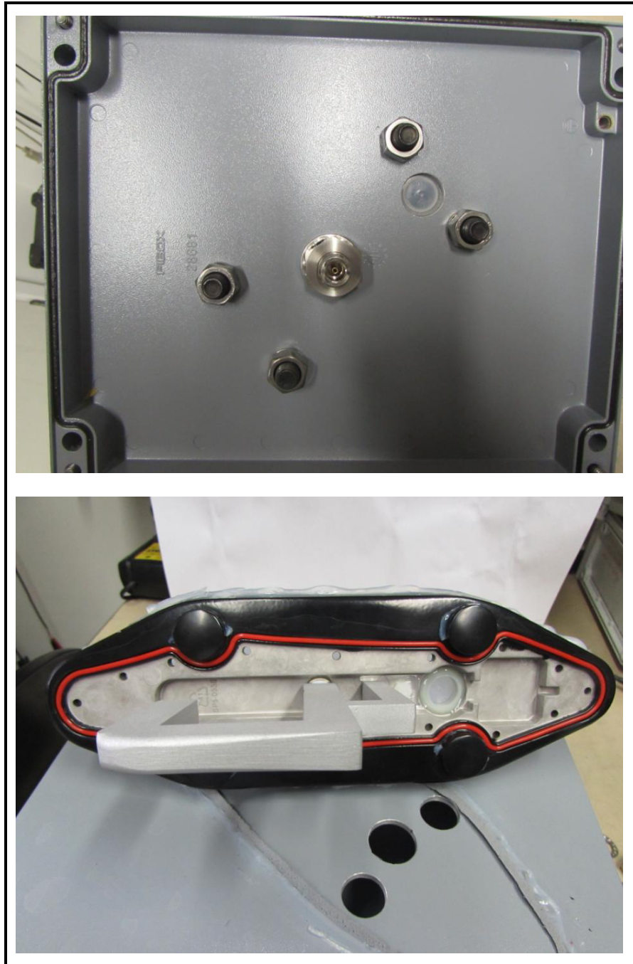
Figure 2: Post Test Photos – IPx9K Water Ingress TRNC[G]
